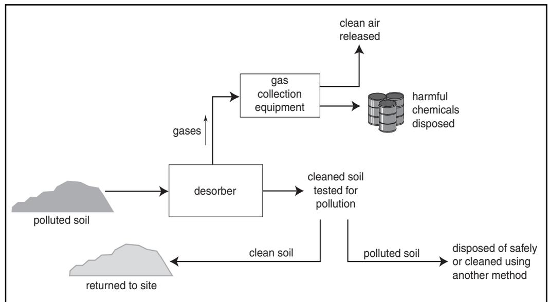
During each step of the process, workers use special equipment to control dust from the soil and collect harmful gases that are released to the air. The polluted gases are separated from the clean air using gas collection equipment. The gases are then changed back into liquids and/or solid materials. These polluted liquids or solids are disposed of safely.
